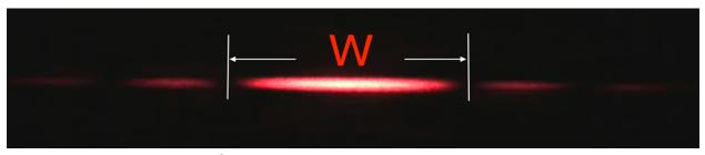
How to measure the width of single slit pattern (W is distance from centers of dark spots)
