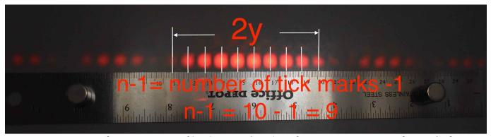
How to measure interference spacing of bright spots (resulting from constructive interference) of a **double slit pattern**
