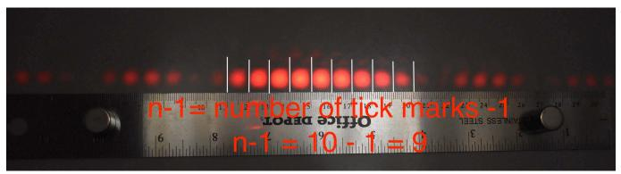
The spacing can also be measured by measuring the center of the dark spots (resulting from destructive interference) of a **double slit pattern.** This tends to be easier to do.
